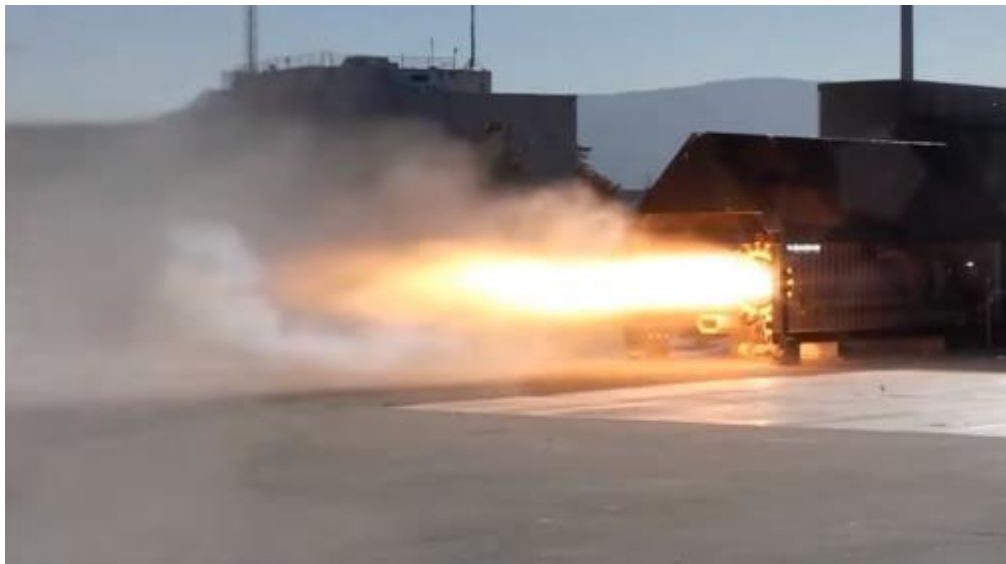
Figure 1.19 A static firing test of Peregrine hybrid rocket motor. 36)
