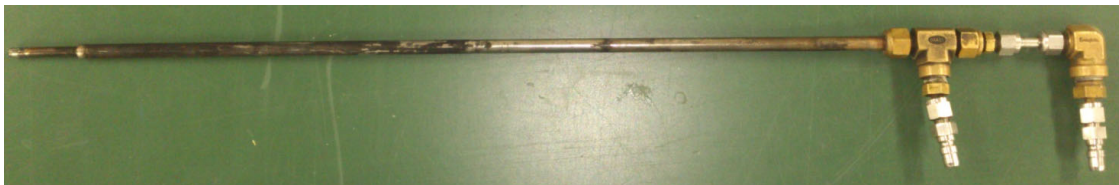
Figure E.12 Launch-stem. (Double pipe)
