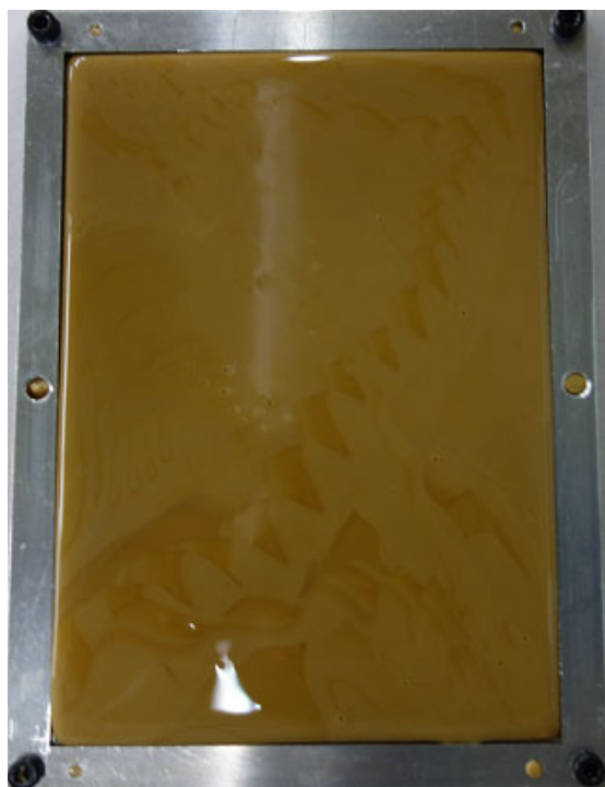
Figure B.3 The melted LT#460 fuel after poured into the molding board.
