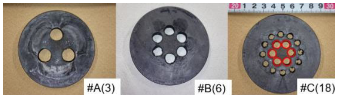
Figure 4.20 Photographs of the baffle plates after the firing test.
