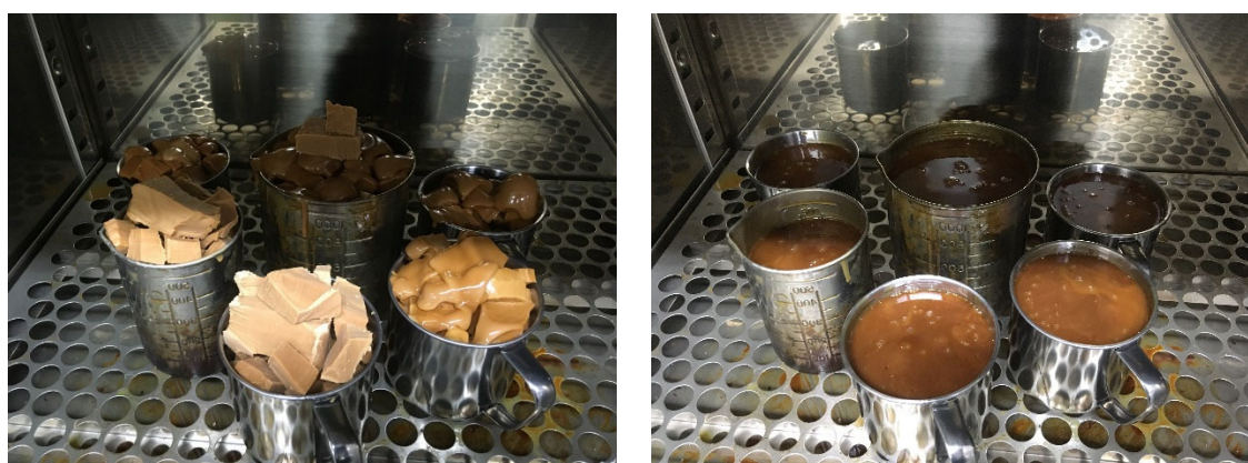
Figure B.11 LT fuels in thermostatic oven. (Left: before, Right: after)
