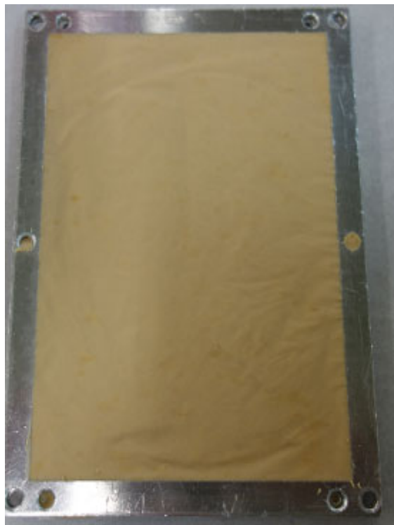
Figure B.4 The solid LT#460 fuel in the molding board.
