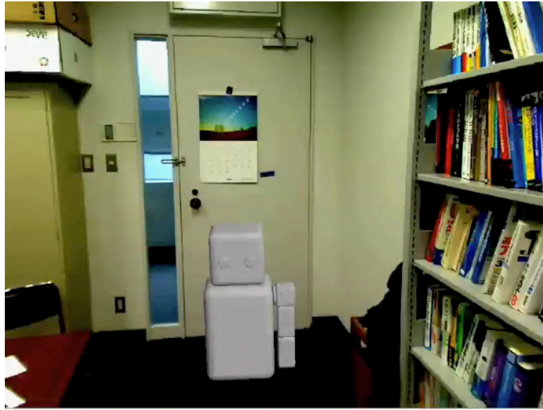
Fig. 3.15: Small robot (height: 900[mm]) displayed using AR for investigating size effects. [宮治 09]
