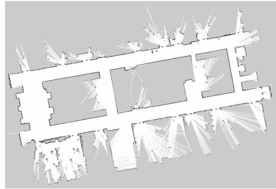
(b) Map built with a robot using an LRF.
